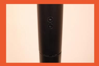
9. Feed front brake wire into frame
