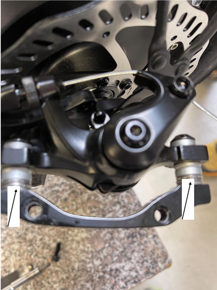
Picture 1. The spacers between the Brake bracket and the brake caliper.
