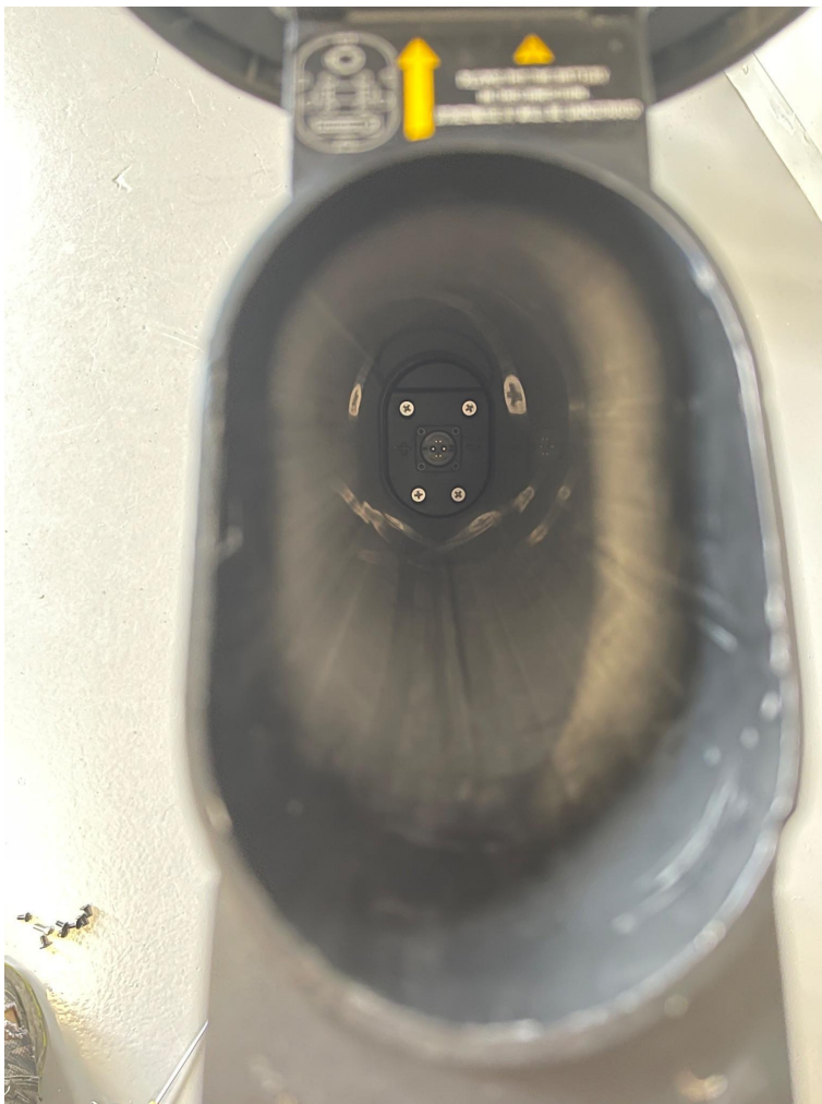
Picture 18. Inside the seatpost. Female Rosenberger connector.
