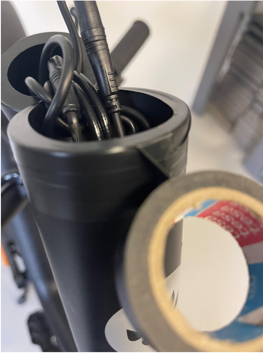
Picture 8. Tape to prevent frame chafing.
