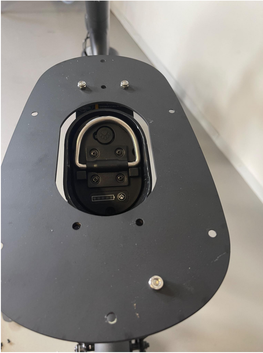
Picture 16. The safety screw for the lock.
