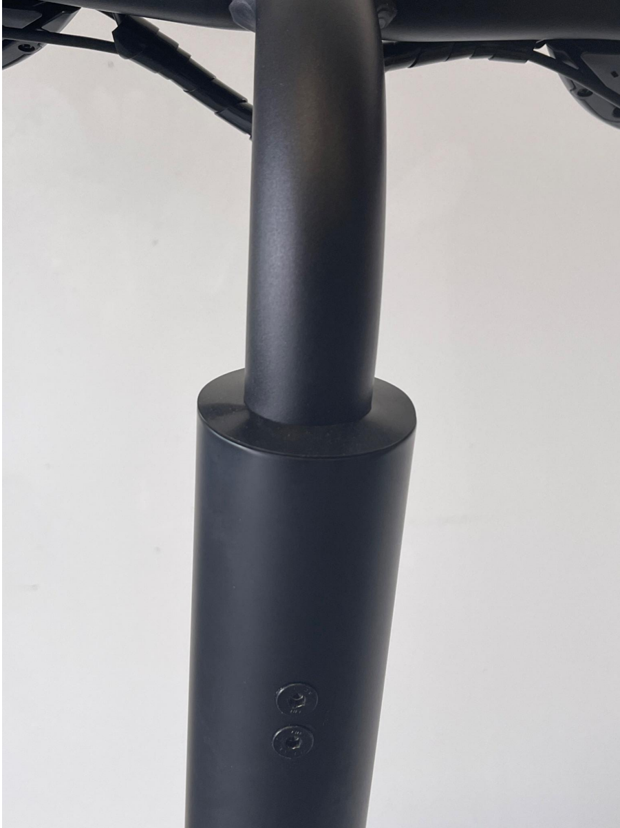
Picture 3. The 2 screws on the top of the steering tube.
