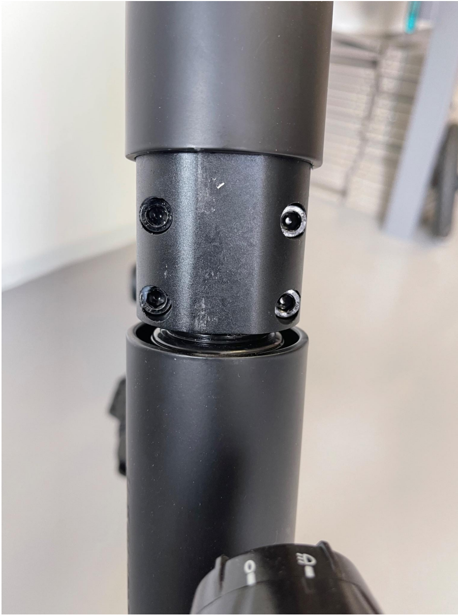
Picture 5. the 4 bolts that you need to unscrew to turn the handlebar alignment with the fork.
