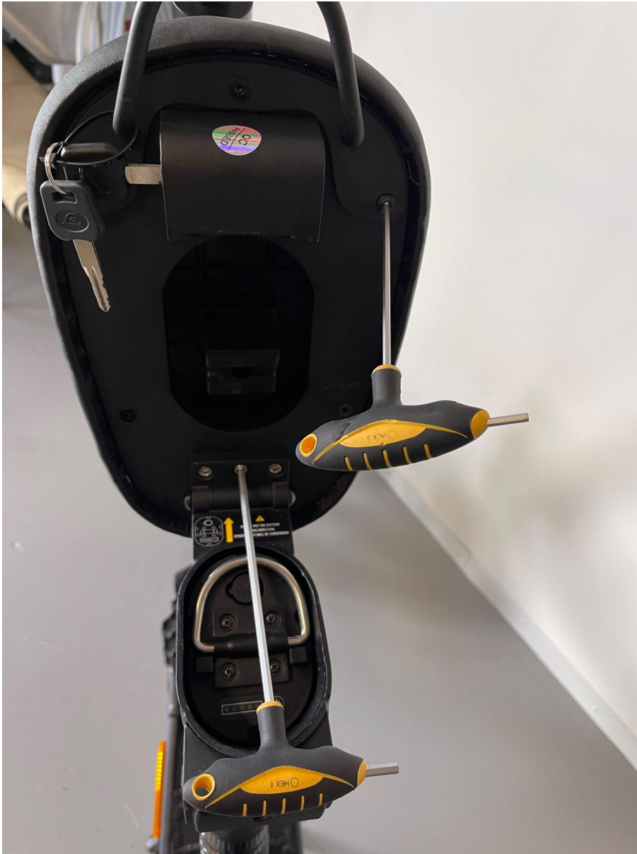
Picture 13. Unscrewing the screws holding the saddle. Don't forget the lowest middle one.
