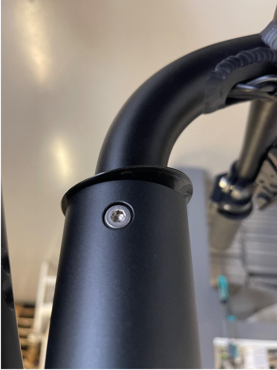
Picture 7. easier to pull on cables if this is unscrewed.
