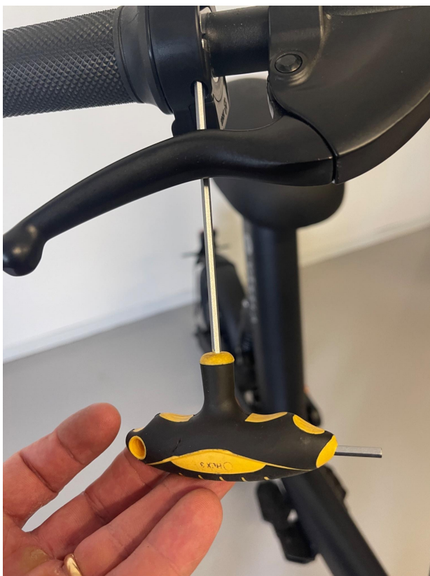
picture 10. How to unscrew the throttle.
