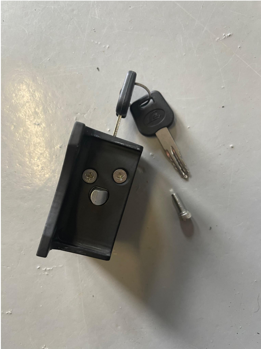
Picture 17. The complete Locking mechanism.
