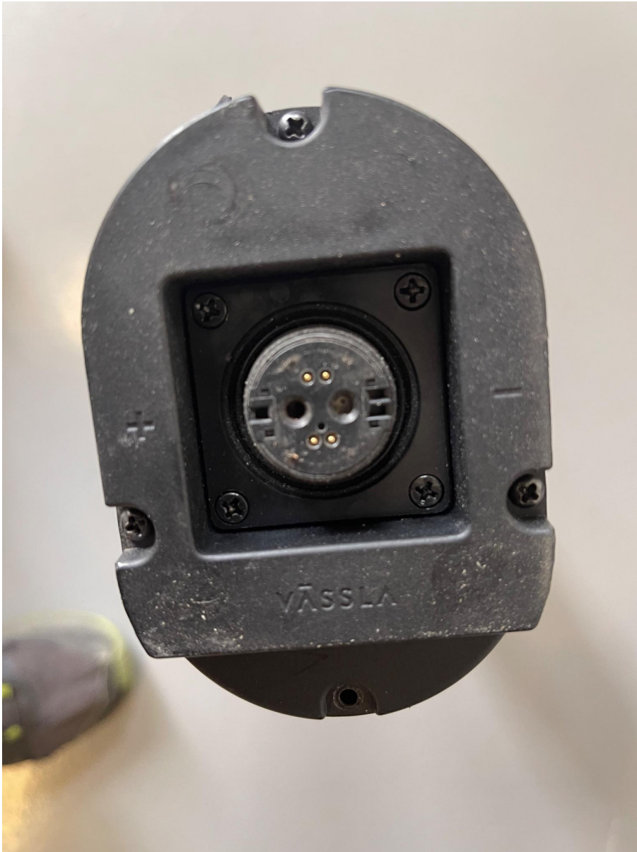
Picture 19. Underneath the battery pack. Male Rosenberger connector.
