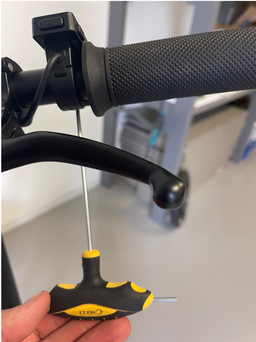
Picture 6. How to unscrew the display.
