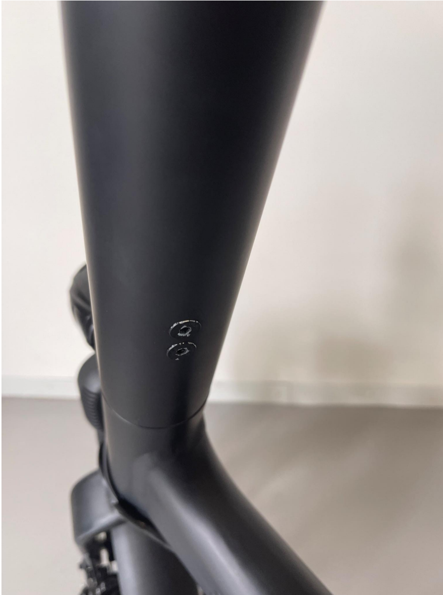
Picture 4. The 2 screws on the bottom rear steering tube.
