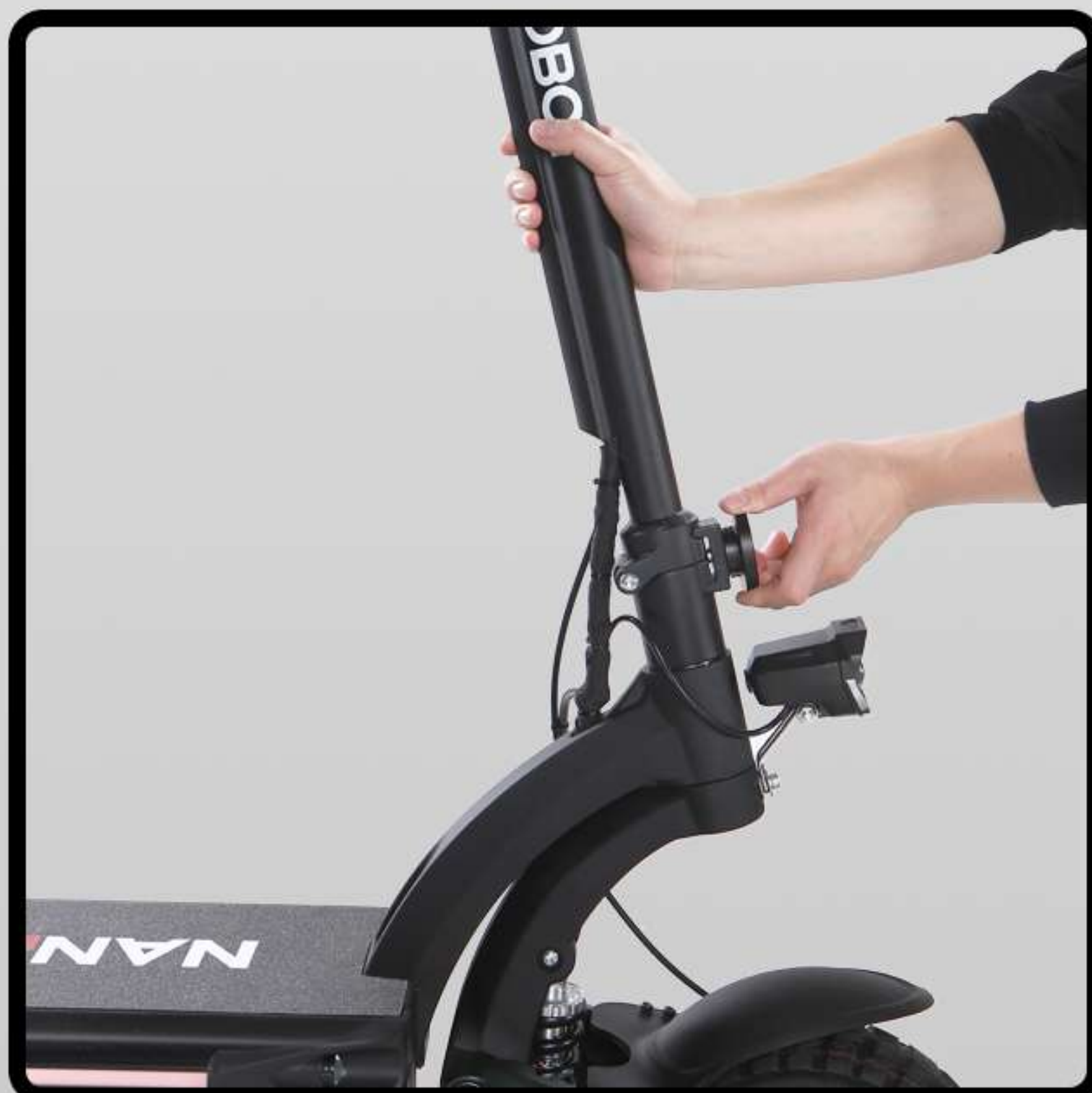
③ Make sure to perfectly align the L-shaped buckle.
