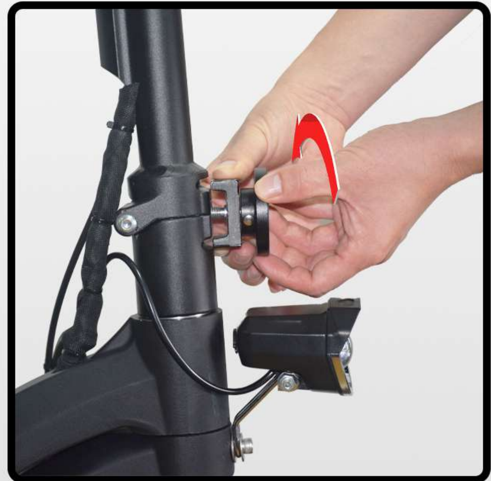
② Align the L-shaped buckle with the grooves, then tighten the folding knob.
