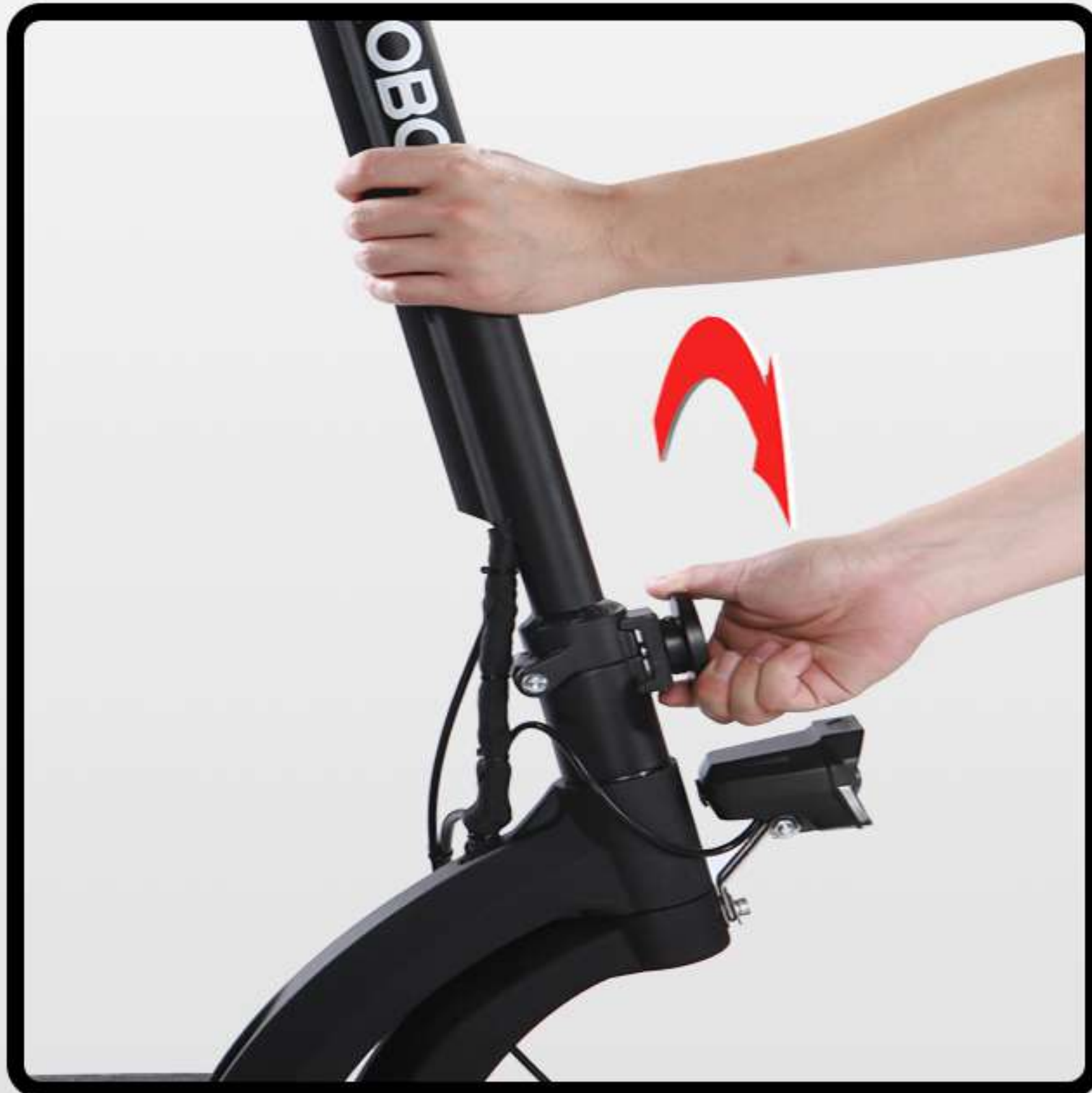
① Loosen the knob in the direction of the arrow.
