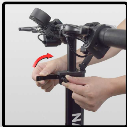
② Loosen the fastening clip in the direction of the arrow
