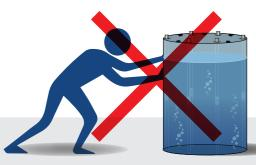
Never drag or move the Flexible Reservoir when full of water. The Flexible Reservoir should be completely drained before it is moved.
