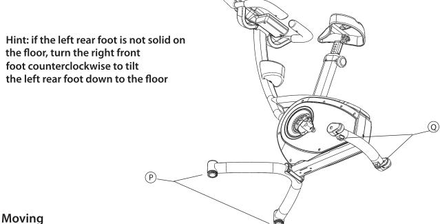
Your C7000i bike is equipped with two transport wheels (R) located on the rear support. Carefully tilt the front of the bike up until the transport wheels in the back make contact with the floor and roll the bike to the desired location. It may be difficult to roll the bike in plush carpeting.
