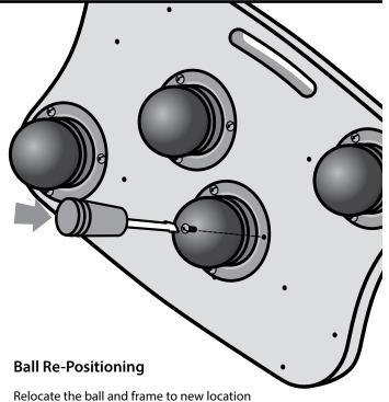
on your balance board and re-attach with the 3 screws.
