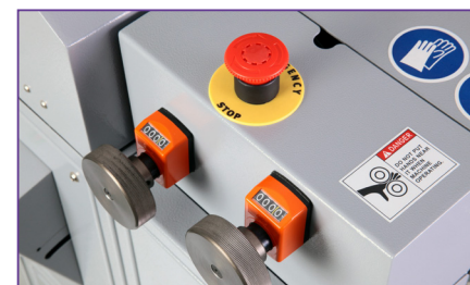
Coating roller gap dials for one-time adjustments
