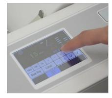
**TOUCH SCREEN** The LED touch screen sets up 18 standard folds automatically at the touch of a button. Up to 12 custom folds can be stored in memory.
