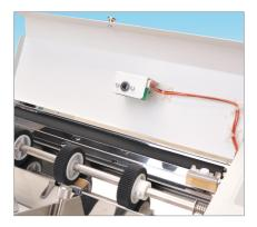
DOUBLE FEED DETECTION The double feed detection sensor prevents mis-folded papers being contaminated to outputs.
