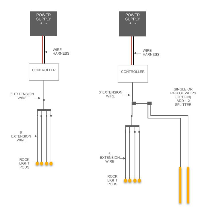
Diagram is example installation. Build outs can vary.
