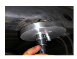
3. The word "WHEEL" with an arrow on the bump stop should be pointing towards the vehicle's wheel. With the bump stop spacer now in place you can reattach the original bump stop to the new bump stop spacer using the bolt and nut (14mm) supplied with the new RAS bump stop spacer.
