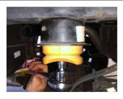
2. Select the correct length bolt for your bump stop from the supplied bolts and drop it into the hexshaped hole on the new bump stop spacer. Align the two roll pins into the holes on the frame using the original O/E bolt and fasten them securely.
