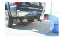
4. Raise the rear of the vehicle with the jack sufficiently to place jack stands on both sides of the vehicle. As the vehicle has rear leaf springs, the ideal place to position the stands is under the front eye of the leaf springs, connected to the fixed shackles, as illustrated. With the floor jack still under the differential, Remove the rear wheels. With the lug nuts now loosened, this will make the removal a lot easier.
