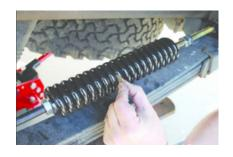
15. Jam one of the two nuts located in the center of the threaded rod hard against the coil spring, then follow with the second nut and jam against the first.
