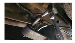
2. Jack the vehicle up and place the jack stands under the frame closest to the front leaf spring connection. Once jack stands are in place using the trolley jack placed under the differential raise it up and remove the nut from the bolt of the rear eye of the leaf spring. Supporting the leaf spring, raise the leaf spring enough to relieve the tension on the bolt and remove the bolt.
