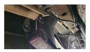
3. Once the bolt is removed, create enough space to allow the hook bracket to be installed over the rear eye of the leaf spring by raising up the frame. Once the hook is centered on the eye of the leaf spring, lower the frame back into position and reinstall the nut and bolt through the shackle and eye of the leaf spring.
