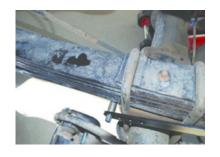
10. Attach the nyloc nut and tighten. The bolt with the spacer must be located directly under the leaf spring. This step is very important.
