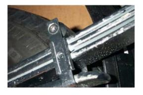
2. This illustration shows the roller removed. In order to remove the counter-sunk hexagon socket head, the bolt must first be removed. The head of the bolt is located on the spare tire side of the vehicle.
