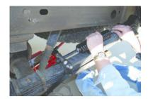
8. The axle connecting brackets have five holes on each side and come with the 12mm bolt, spacer, and nyloc nut, located through the end holes in the bracket. The nyloc nut has only been turned on hand tight. Next remove the nut, bolt, and spacer. The bracket should now hang astride the leaf spring pack and U bolts.
