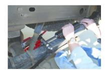
8. This kit comes with extension brackets. Please see page 5 for extension bracket instructions. The axle connecting brackets have five holes on each side and come with the 12mm bolt, spacer, and nyloc nut, located through the end holes in the bracket. The nyloc nut has only been turned on hand tight. Next remove the nut, bolt, and spacer. The bracket should now hang astride the leaf spring pack and U bolts.
