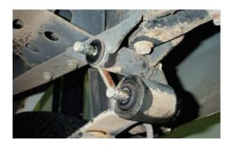
4. Position the eye bracket over the eye of the leaf spring and replace the side of the shackle that was removed then secure the two nuts. Follow these steps for both sides.
