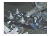
12. Before adjusting the coil spring to the correct tension, check to see that the eye bracket is in the center of the spring eye.
