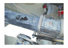
10. Attach the nyloc nut and tighten. The bolt with the spacer must be located directly under the leaf spring.
