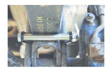
15. Before adjusting the coil spring to the correct tension, check to see that the eye bracket is in the center of the spring eye.
