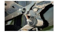
9. Position the eye bracket over the eye of the leaf spring and replace the side of the shackle that was removed. Secure the two nuts and repeat on the other side of the leaf spring.
