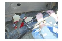
12.The axle connecting brackets have five holes on each side and come with a 12mm bolt, two washers, a spacer, and nyloc nut, located through the end holes in the bracket. The nyloc nut has only been turned on hand tight. Next remove the nut, bolt, spacer, and washers. The bracket should now hang aside the leaf spring pack and U bolts.
