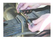
13. With the axle bracket now in position under the leaf springs, insert the connecting bolt and spacers. Make sure the flat head of the bolt is facing the shock as in structed on page 3.
