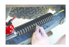
18. Jam one of the two nuts located in the center of the threaded rod hard against the coil spring, then follow with the second nut and jam against the first.
