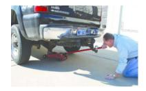
4. Raise the rear of the vehicle with the jack sufficiently to place jack stands on both sides of the vehicle. As the vehicle has rear leaf springs, the ideal place to position the stands is under the front eye of the leaf springs, connected to the fixed shackles, as illustrated. With the floor jack still under the differential, Remove the rear wheels. With the lug nuts now loosened, this will make the removal a lot easier.
