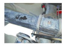
14. Attach the nyloc nut and tighten. The bolt with the spacer must be located directly under the leaf spring.
