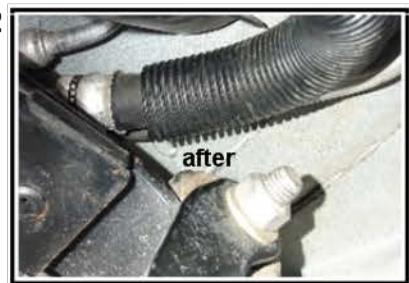
2) ILLUSTRATION SHOWING HOW THE LINES LOOK AFTER THEY HAVE BEEN RE LOCATED. THE ROADMASTER KIT CAN NOW BE INSTALLED WITHOUT INTERFERING WITH THE REAR A/C AND HEATER LINES.
