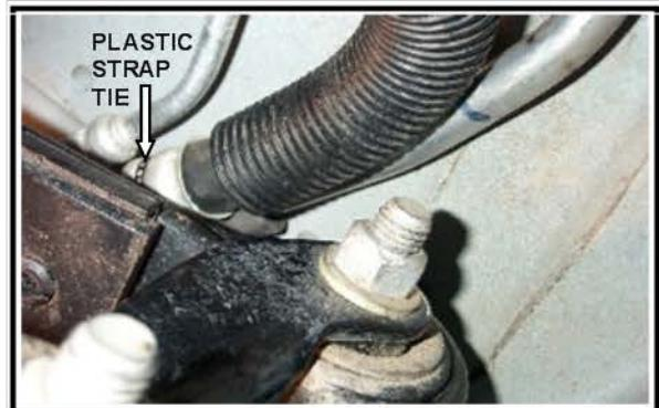
9) ILLUSTRATION SHOWING THE TWO LINES NOW AWAY FROM THE LEAF SPRING EYE. NOTE PLASTIC STRAP TIE HOLDING BOTH LINES TOGETHER.
