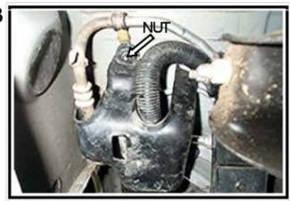
3) ON SOME VANS GM HAS FITTED A PLASTIC COVER LOCATED ON THE REAR DRIVERS SIDE. THIS COVER MUST FIRST BE REMOVED BEFORE THE LINES CAN BE REPOSITIONED. THE COVER IS FASTENED TO THE UNDERSIDE OF THE VAN WITH ONE NUT, LOCATED ON A STUD ON THE UNDERSIDE OF THE FLOOR PAN. THIS STUD IS ALSO USED TO HOLD THE SUPPORT BRACKET FOR ONE OF THE A/C LINES. THERE ARE ALSO TWO PLASTIC PUSH FASTENERS HOLDING THE COVER, THAT MUST ALSO BE REMOVED.
