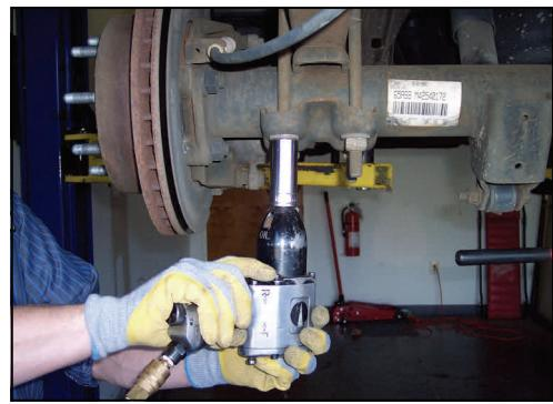
**2) WITH THE AXLE NOW WELL SUPPORTED, REMOVE THE TWO U/BOLT NUTS AS SHOWN IN ILLUSTRATION IN (3)**
