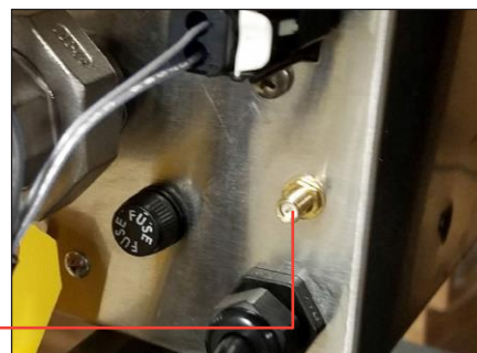
Figure 6.6 – Attach antenna cable
