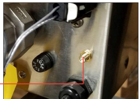
Figure 6.10 – Attach antenna cable
