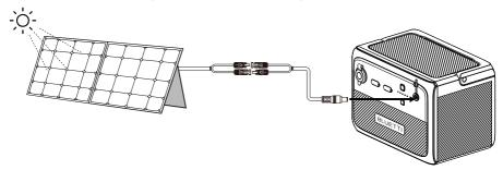
*Warning:* The open circuit voltage of solar panels cannot exceed 28V, otherwise it will damage the device.(Note:This is not covered in the warranty.)
