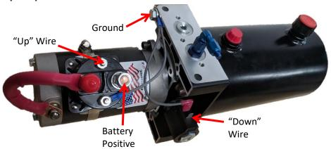
The pump has 4 total electrical connections; positive, negative and two signals.
