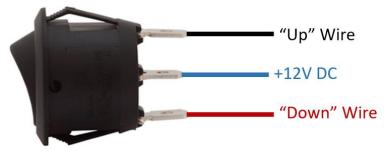
Note: If a custom pump control system is to be used rather than a switch, it simply needs to supply 12v to the wire corresponding to the desired direction of motion.
