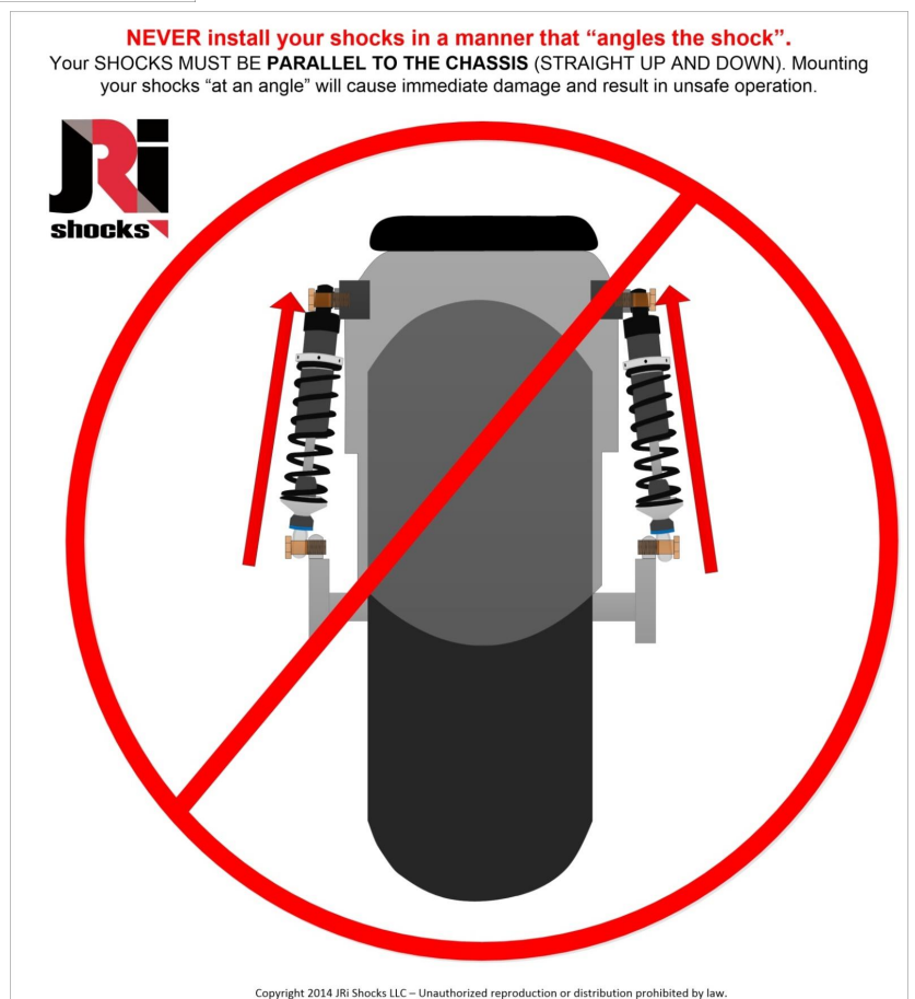
Figure 7 – DO NOT INSTALL SHOCKS AT AN ANGLE
