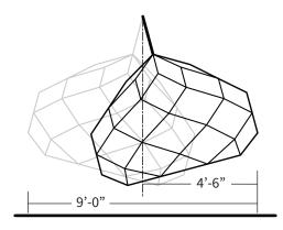
Typical minimum clearance dims shown. Actual amount of swing depends on length of rigging to overhead anchor.
