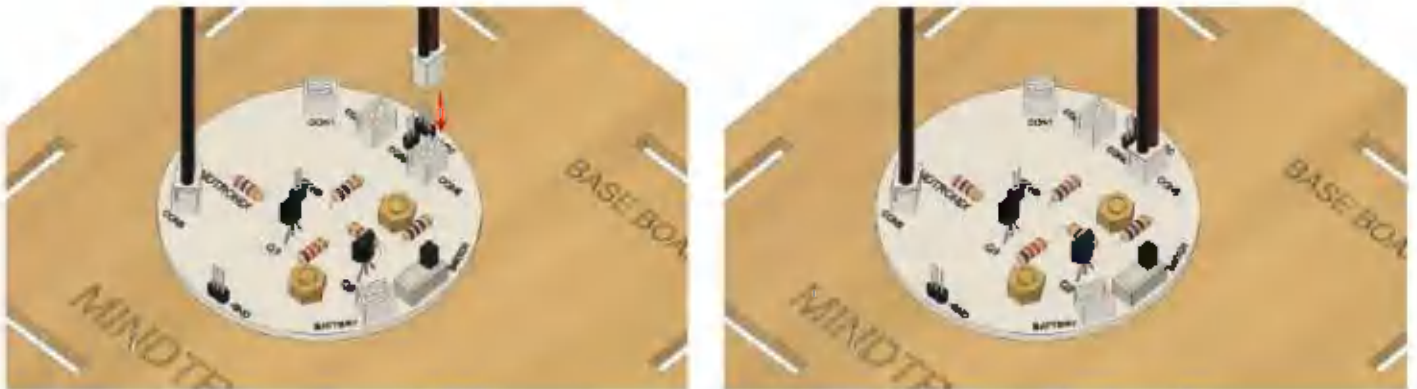
15. Insert the Buzzer's extension cable in to the CON6 of main board
