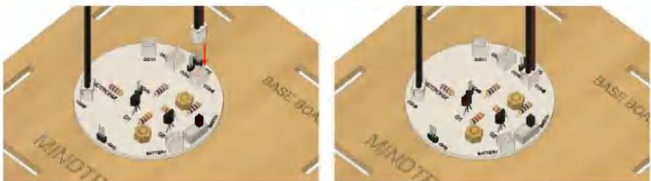
16. Connect the LED's extent ion cable in to the CON6 of main board
