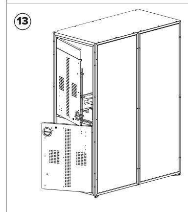
Attach the lower and upper doors with (8)  $\#12 \times 3/4$ " self-drilling screws. Pilot holes are present but may be partially filled with zinc. Note the upper door has an extra top panel.
