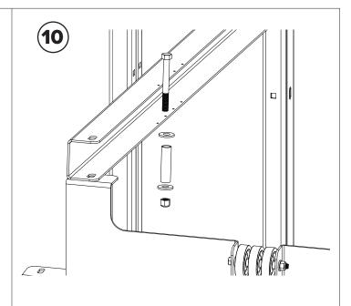
Secure the front of the (2) Dero Decker tracks with (1)  $3/8" \times 3.5"$  hex bolt, washers, and lock nut.
