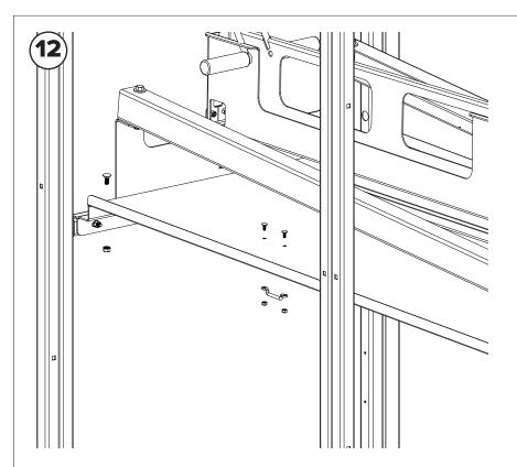
Attach the drip tray with (4) 5/16" x 3/4" carriage bolts and lock nuts. Note that the small holes in the drip tray are oriented towards the front of the locker. Attach the spring mount with (2) #10 x 1/2" carriage bolts and locknuts.
