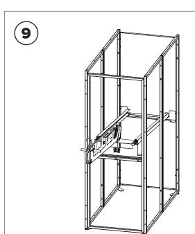
Insert the Dero Decker tray assembly into the tracks.
