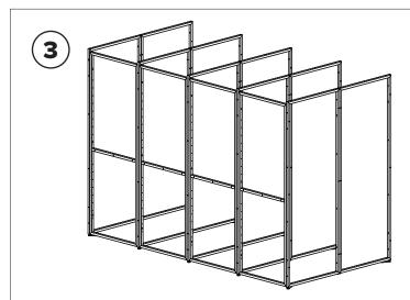
If a modular row of lockers is being assembled, continue attaching frame assemblies and door frames. Level the assembly with the leveling feet and secure them to the ground with 3/8" diameter anchors.
