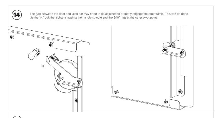
If any twist needs to be taken out of the door, loosen the (10) #10 locknuts, set the door, and re-tighten.
