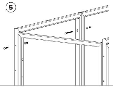
Attach the frame panels to the side positions in frame assembly with (4) 5/16" x 2.25" and (4) 5/16" x 4" carriage bolts, washers, and lock nuts. Continue adding side frame panels if assembling a modular row. The (3) bolt holes at the bottom of the panels are not used. The (3) bolt holes at the top of the panels will be used later.
