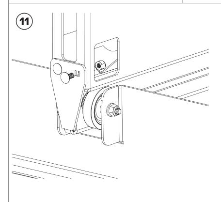
Feed the wheel guide under the center wheel and attach to the tray with (4) 1/4" x 5/8" carriage bolts and lock nuts.
