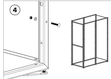
Attach (1) frame panel to the rear position in frame assembly with (4) 5/16" x 2.25" carriage bolts, washers, and lock nuts. Note the center bolt position will be left open for now. Continue adding rear frame panels if assembling a modular row.
