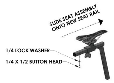
**4.** Attach the training bar assembly to the seat rail using the supplied 1/4" hardware as show below.
