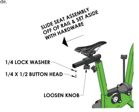
**2.** Loosen the adjustment knob on the main frame and remove the seat rail assembly from the main frame.
