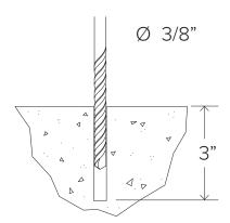
Drill 3/8" diameter holes 3" deep into surface. Make sure the holes are at least 3" away from any cracks in the base material.
