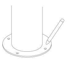
Attach the Cycle Stall segments on street with the supplied  $3/8" \times 2.75"$  carriage bolts, and move assembled unit into place.
