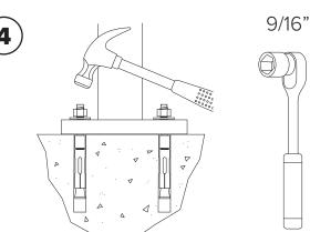
Thread nuts onto anchors, leaving approximately 1/4" of the anchor protruding, and tap into surface. Tighten nuts down to secure rack.
