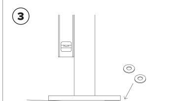
Place rack (and washers to level rack if necessary) over holes.
