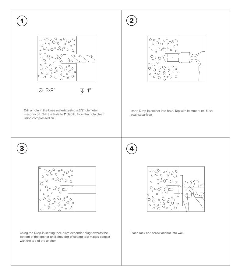
Installation Concrete Block Wall
