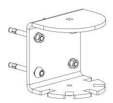
For **solid concrete**, hammer in the wedge anchors through the base and into the wall. Tighten (2) of the hex nuts and replace the other (2) hex nuts with Penta nuts and tighten. For **hollow concrete**, hammer the sleeve anchors directly into the wall. Tighten all (4) nuts until the anchors are set. Remove the nuts and place the base over the anchors. Tighten (2) hex nuts on the anchors and tighten (2) Penta nuts on the remaining anchors.
