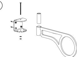
Place the pin through the arm hinge and secure to the base with a 3/8" x 6.5" carriage bolt, 3/8" washer, and Penta nut.
