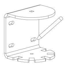
Place the Alley Rack base on the wall where it's to be installed with the top of the base 32" from the ground. Use the base as a template and mark the wall through the (4) mounting holes.
