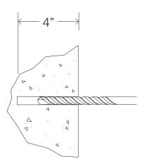
For **solid concrete**, drill 3/8" diameter holes about 4" deep. For **hollow concrete** walls or hollow concrete block, drill 1/2" diameter holes through the wall. If the wall type is **not known**, drill 3/8" diameter holes. If the wall is solid then stop and use 3/8" wedge anchors. If the wall is hollow then use the 3/8" diameter holes as pilot holes for a 1/2" drill.
