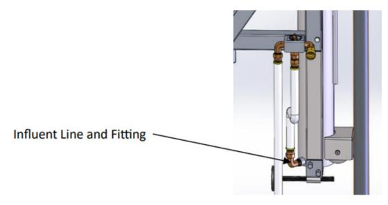
4. Remove Small hose and fitting from cylinder. Replace with new fitting and hose.
