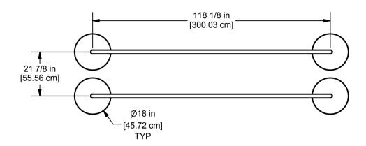
CONCRETE REQUIRED: 0.44 CUBIC YARDS [0.33 CUBIC METERS]
