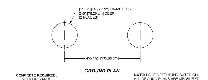
.20 CUBIC YARDS [.15 CUBIC METERS] **NOTE:** HOLE DEPTHS INDICATED ON ALL GROUND PLANS ARE MEASURED FROM THE FINISHED SURFACE. SEE DETAIL 321. ALL FOOTING DIMENSIONS ARE BASED ON LEVEL FINISHED SURFACE.
