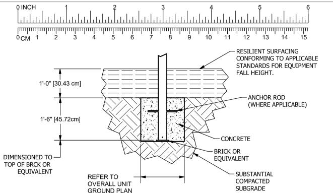
SHOCK ABSORBING PROPERTIES OF SURFACING MATERIALS M,AY VARY. IF YOU DETERMINE THAT LESS THAN 1'-0" [30.48cm] OF SURFACING IS REQUIRED, MAKE UP THE DIFFERENCE IN ELEVATION WITH EARTH BEFORE APPLYING SURFACING.
