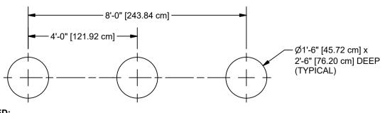
CONCRETE REQUIRED: .30 CUBIC YARDS [.24 CUBIC METERS]
