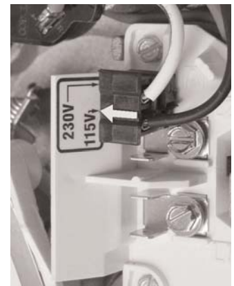
Figure 5B -Voltage Change Plug Set for 115 Volts
