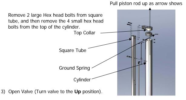
Pull on piston rod until the Top collar just comes out of cylinder tube. Slide top collar off of piston rod.
