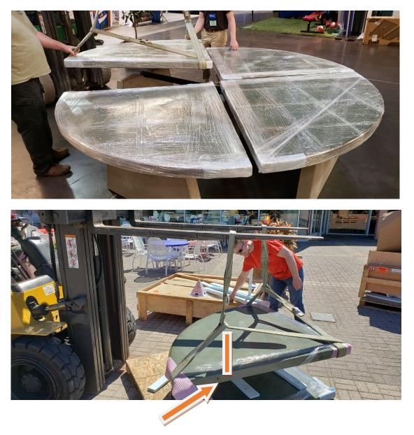
Pick point should be between 15" and 16" from the rounded edge towards the square corner for optimum balance.
