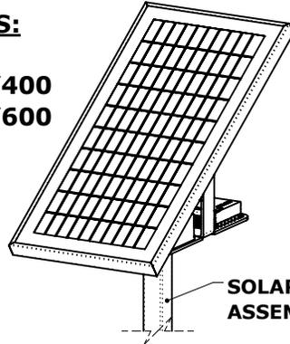
**TO INSTALL THE 24V SOLAR PANEL, USE THE MOUNTING BRACKET (INV01879) AND THE (02) TWO 5" BUTTON HEAD BOLTS, FLAT WASHERS, AND LOCK NUTS. PASS THE BOLTS THROUGH THE BRACKET AND TO THE OPPOSITE SIDE OF THE MAIN FRAME.**
