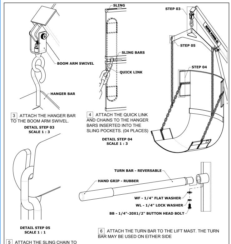
NOTE: BE CAREFUL NOT TO OVERTIGHTEN BOLTS. OVER-THE HANGER BAR. ADJUST THE CHAIN TO THE HEIGHT THAT WORKS SAFETY OF YOUR LIFT BEST FOR YOUR NEEDS.
