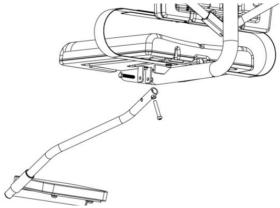
Tighten the bolt until the flat washers are snug, and then back off until the footrest pivots freely. Adjust footrest to desired height by installing and adjusting 3/8" - Button Head Bolt through footrest assembly coupling nut. Use 3/8" Hex Nut to lock position setting.
