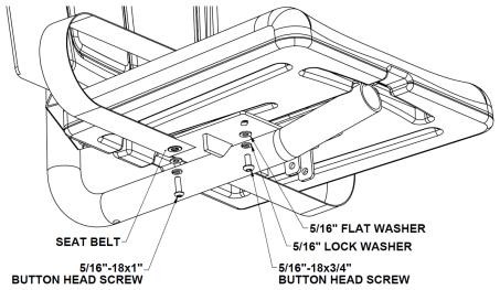
Note: When attaching the seat belt use 5/16"-18 x 1" as shown below:
