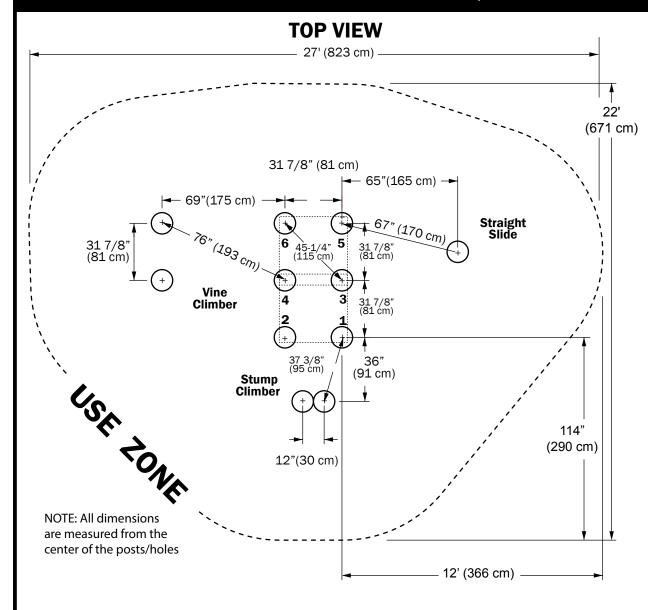
**IMPORTANT:** Never install play equipment over hard, unresilient surfaces such as asphalt, concrete or compacted earth. It is the owner's responsibility to ensure the "minimum area required" contains an appropriate amount of resilient material to cushion accidental falls.
