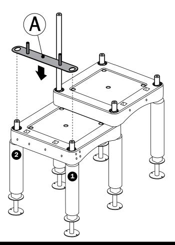
1. Place Climber Handhold Bracket(A) onto top surface of Deck between Posts #1 and #2.
