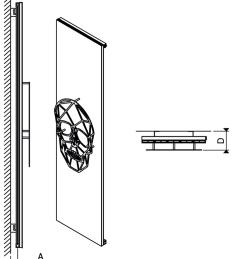
Max. working pressure 10 bar Max. working temperature 95 °C Connections 1/2" Section depth 48 mm Pipe center W + 90 mm
