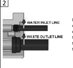
Place water inlet and drain outlet pipes on the corresponding holes on the toilet body. Mark the pipes on the point where they meet the toilet body. 3
