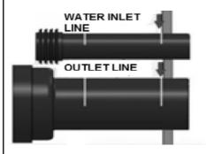
Water inlet and drain outlet pipes are placed into the installation holes on the wall. Mark the points on the both pipes where they meet the wall.
