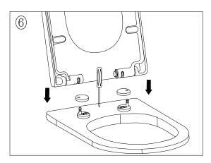
6. Tighten the screw and fix the cover and seat after covering the two caps on the hinges.
