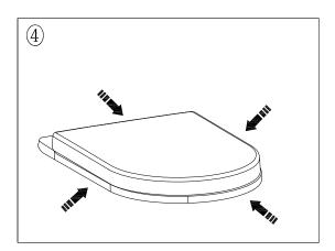
4. Adjust the S&C to appropriate position to match the pan well.
