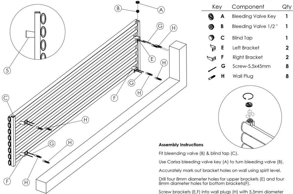
Hang radiator by sliding the bosses on the back of the radiator into brackets (E,F).
