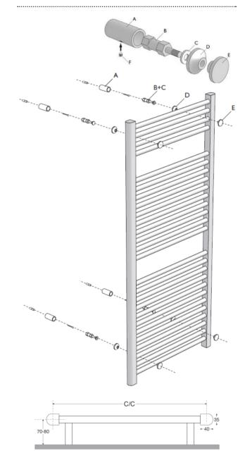
Tapping centres (C/C) for Hugo2 radiators are 40mm less that the width of the rail and 70mm out from the wall
