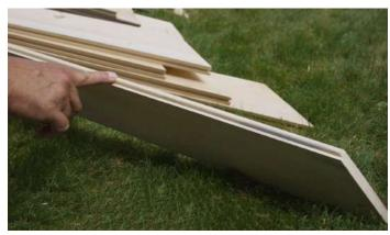
The roof boards are tongue and groove.
