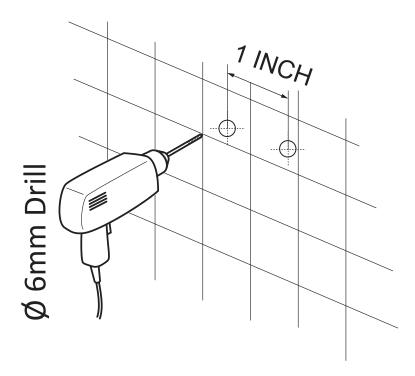
**IMPORTANT** Before drilling any holes for the shower panel brackets, ensure there are no hidden cables or pipelines aligned with the desired drilling position.
