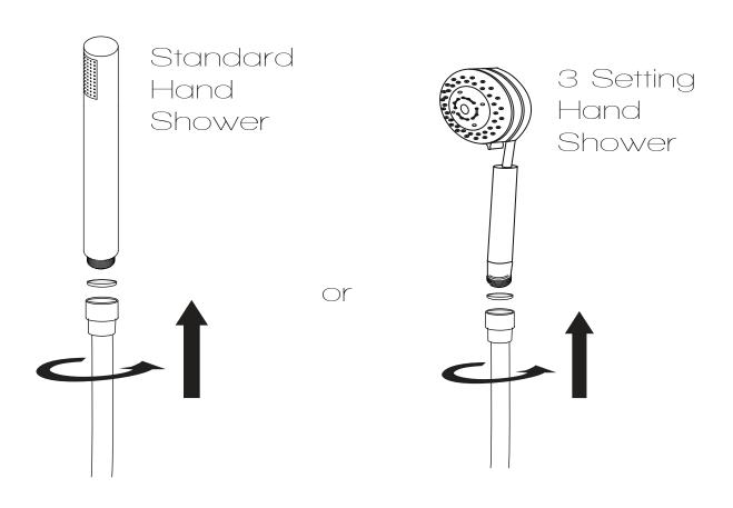
**Step 2A** Finally, install the shower wand to the hose, as shown.
