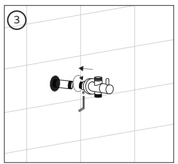
Screw diverter body onto nipple and secure with set screw.
