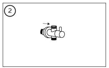
Slide escutcheon onto diverter body
