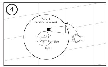
Remove the tape cover and apply a good amount of glue on the mounting hardware. Place the handshower holder, hold in place for a few minutes and let the glue cure for about 48 hours. DO NOT place handshower until glue is fully cured.
