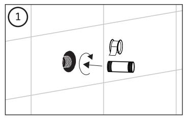
Determine what size nipple is needed. Apply plumbers tape to nipple and connect to your plumbing  $\,$
