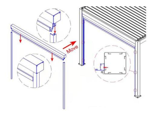
\*\*\* Note, plan which side you want the screen to align to before screwing the side rail. \*\*\*
