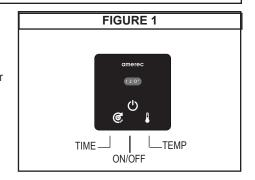
If a K3 is installed without a K73: The K3 control may be mounted inside or outside the steam room, approximately 4 feet up from the floor. A second K3 control may be installed so one is inside and the other outside the steam room. Either control my be used to control the steam bath. Note: when a K3 controls the steam bath without a K73 installed, a separate temperature sensor must be installed in the steam room.
