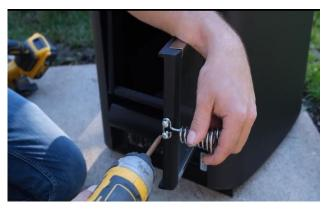
Fasten the stove handle onto the stove door With the screws provided.
