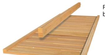
Flip over flat floor, measure the center and place the bottom support in the center.
