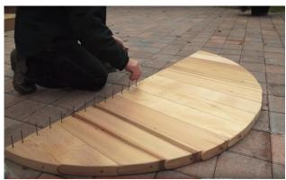
Line up the cove pieces starting with the smallest pieces on the end and working towards the middle forming a semi circle.
