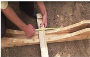
Center the stave onto the cradle and measure 5  $\frac{1}{2}$ " (14cm) from the end of the stave to the edge of the cradle.
