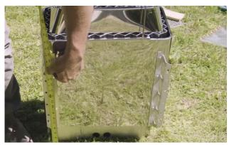
Measure the height of the mounting holes and add 6". (152mm)
