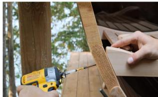
Use a 2  $\frac{1}{2}$ " (64mm) screw to fasten the front and the back of the porch seat screwing through the side stave into the seat supports.
