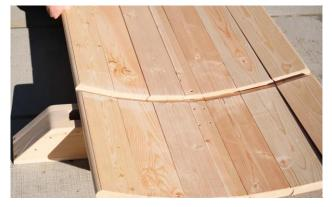
Place 3 staves on either side of the bottom stave and align the grooves.
