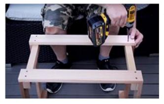
Screw heater guard support to either side using  $(2) - 1 \frac{1}{2}$ " (38mm) screws per side.
