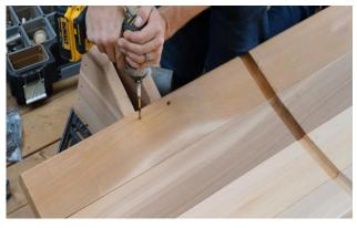
Place 2- 2 ½" (64mm) screws into the 3<sup>rd</sup> stave on either side lining up with the cradle underneath.
