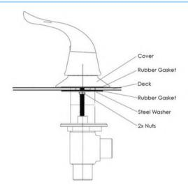
**1.** Unscrew the 2 nuts securing the steel washer and rubber gasket. In this order, remove the steel washer and rubber gasket, place your lever on the deck, replace the rubber gasket and the steel washer. Firmly secure the 2 nuts to hold the fixture in place.
