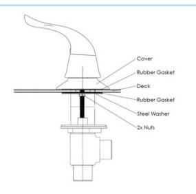
Unscrew the 2 nuts securing the steel washer and rubber gasket. In this order, remove the steel washer and rubber gasket, place your lever on the deck, replace the rubber gasket and the steel washer. Firmly secure the 2 nuts to hold the fixture in place.
