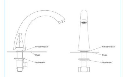
2. Unscrew the washer nut and place the rubber gasket and spout above the deck. After, secure the washer nut from underneath the deck.
